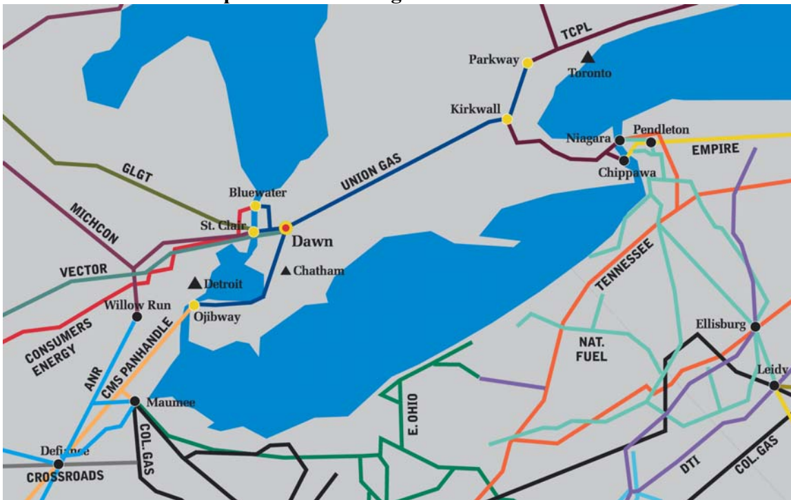
Figure 4 Pipelines Connecting to the Union Gas Hub
