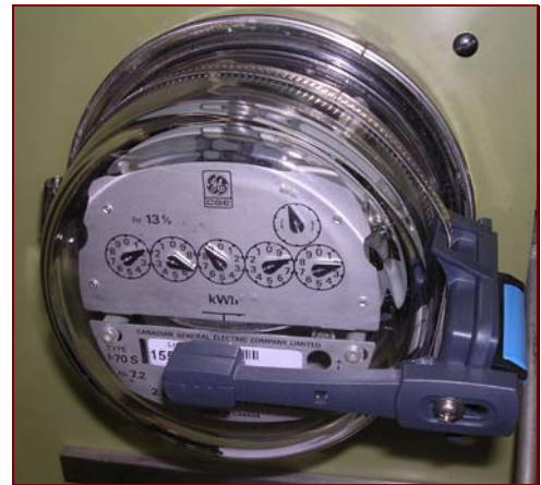
Figure 4-4, Detection Unit Installed on Electromechanical Revenue Meter
