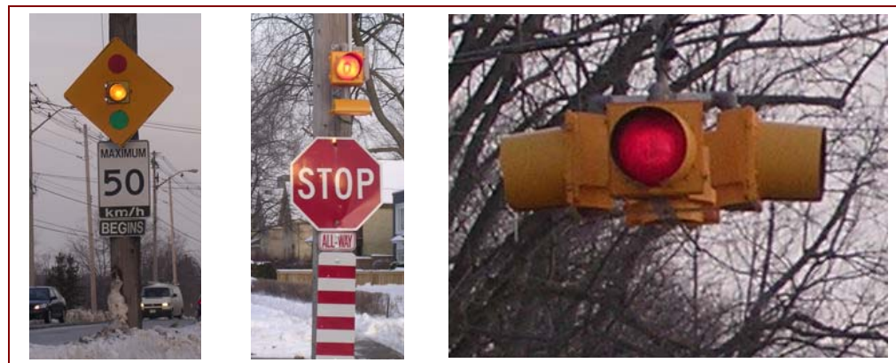
Figure 3-7, Examples of Continuously Flashing Signals
