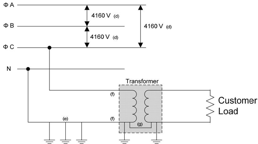
**Figure 2 - Distribution Configuration after the 1930s**
