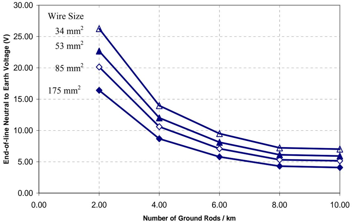
**Figure 7 – NEV for Various Number of Ground Rods - System Voltage = 12.5 kV**
