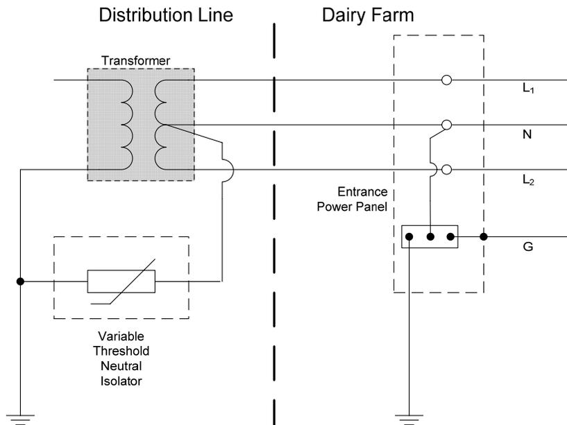
**Figure 11 – Variable Threshold Neutral Isolator Installed on Utility Pole**
