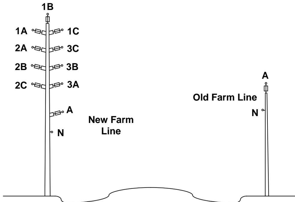
**Figure 13 - Layout of a Wind Farm Collection Line and Parallel Lines for Farm Services**
