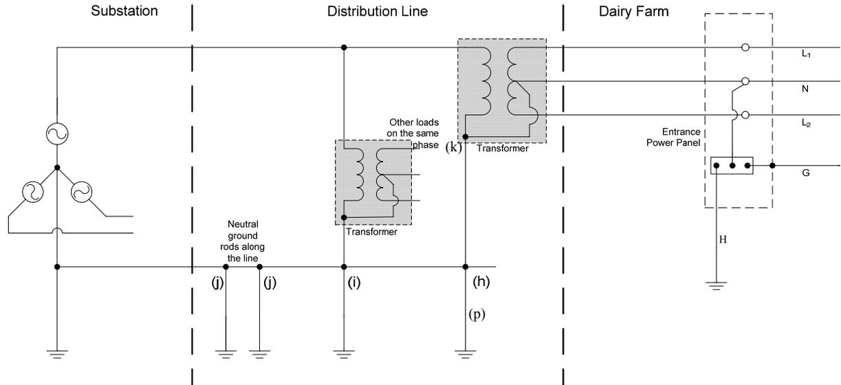
**Figure 4 - Electrical Diagram of a Power Distribution Network**
