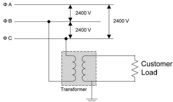
**Figure 1 - Distribution System Configuration Before 1930**
