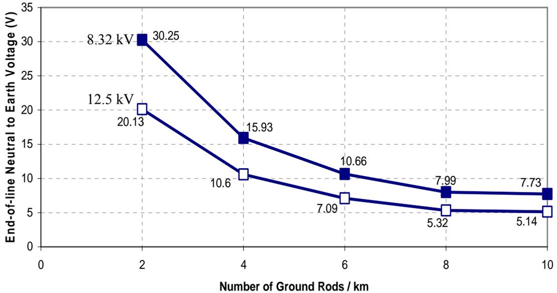
**Figure 6 – NEV by system voltage and grounds per km
