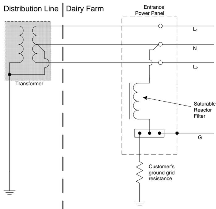
**Figure 12 – Saturable Reactor Filter Installed at the Entrance Power Panel**
