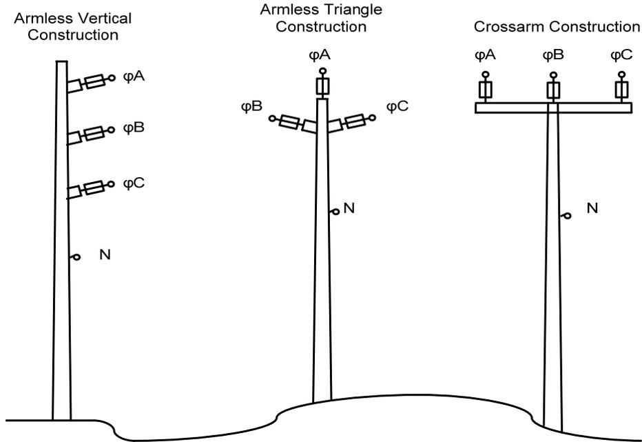
**Figure 8 - Typical Pole Configurations**
