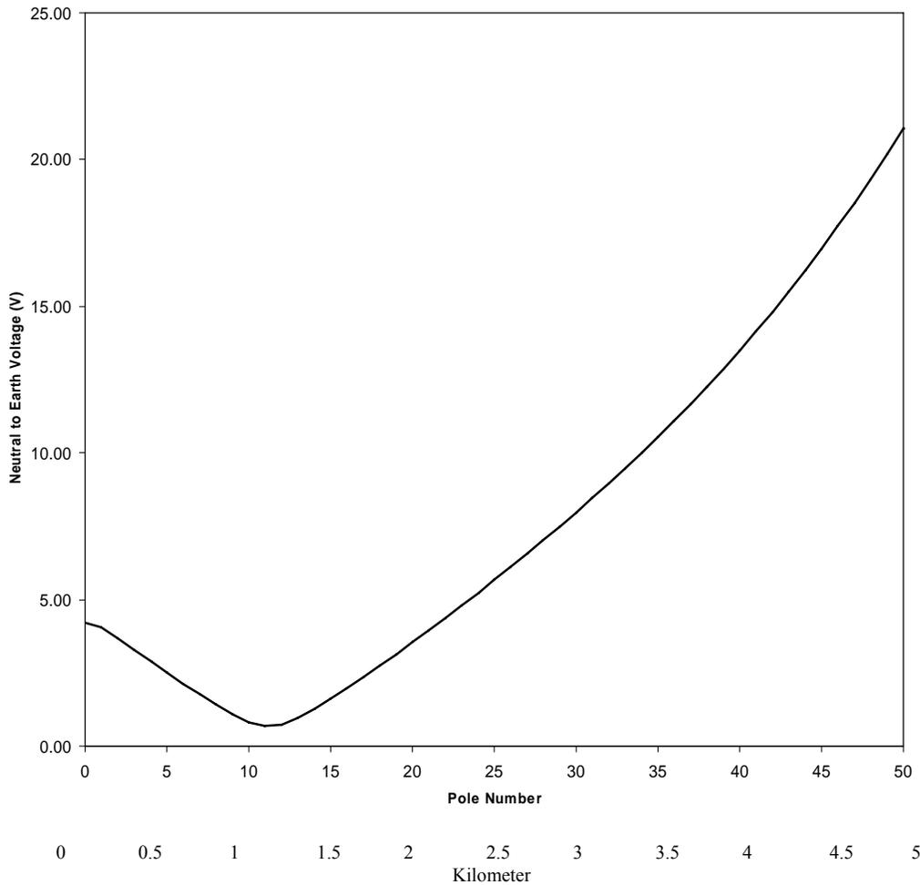
**Figure 9 – Neutral to Earth Voltage for a Balanced Load With Armless Pole Configuration**
