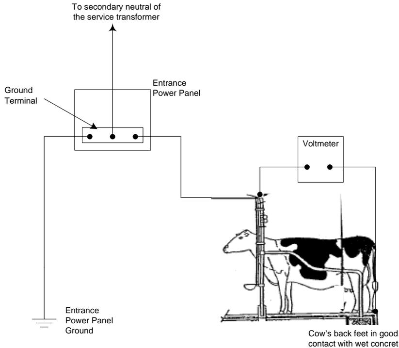
**Figure 3 – Stray Voltage Measurement**
