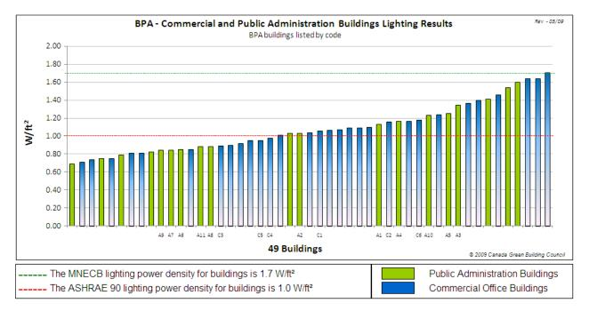
Chart showing results of lighting power intensity across 49 office buildings using similar technology. Most installations use T8 lamps with several T12 installations mixed across the middle. In fact, the poorest performing lighting technology on the far right is in a retrofitted building that replaced T12 lamps with T8s. Note that industry good practice is considerably better than either Canada's Model National Energy Code or the current ASHRAE standard.
