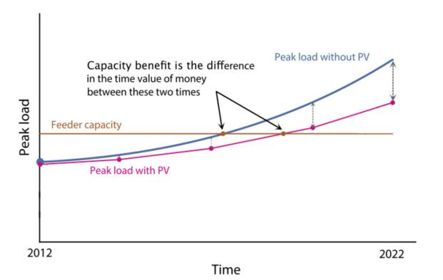
The deferral value would be greatest where the current peak load is near the capacity of the distribution feeder and where the solar is coincident with the peak load on the feeder
